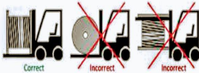
Fig 3.2.9: Unloading of cables
